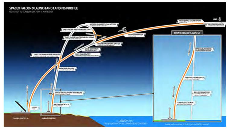
**Figure 2:** The diagram of the flight profile of the Falcon 9 with a landing back at the Kennedy Space Center shows that if the payload is not too heavy, the booster can be flown back to the launch area and land on solid ground. The engine burn to slow the booster down uses three of the seven Merlin engines. Landing back at Kennedy saves time and costs since the drone ship does not have to be taken out to the landing zone and then returned.
