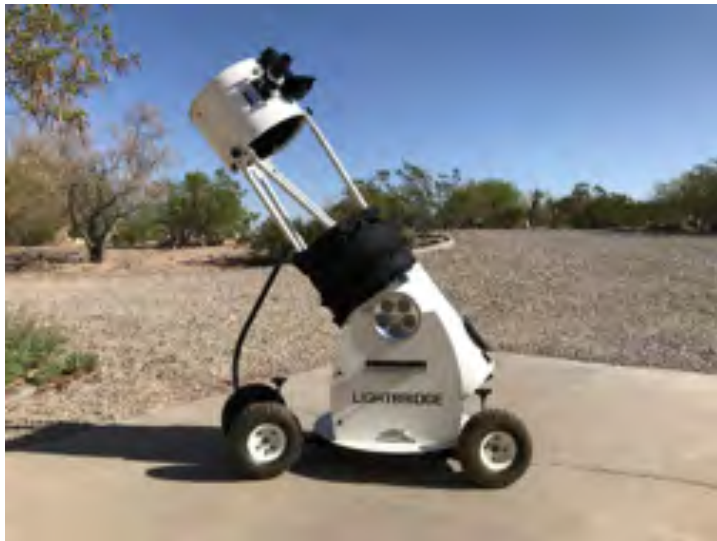
Figure 1: Assembled Meade 12 inch f/5 telescope with black cloth partially covering truss, loaded onto a wheeled cart.
