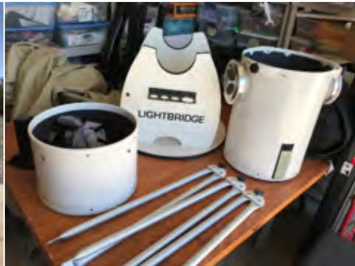
Figure 2: Telescope disassembled, showing front optical tube, mount, rear optical tube, and the three truss bars.
