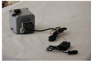
Cooler assembly with 12V connector and switch
