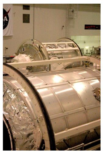
The picture at left shows the Tranquility Node and cupola, that last segments to be added to the American side of the station in order to reach "core complete" status. The other nodes on the shop floor are for the Russian side.
