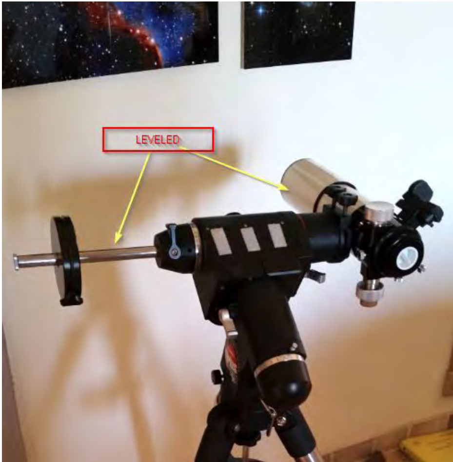
Figure 8: Telescope leveled on east side of mount during alignment.
