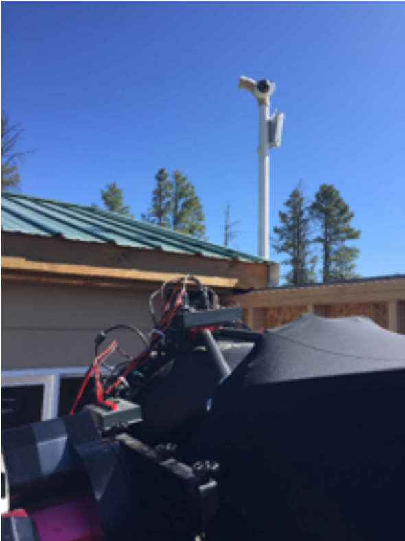
Simple to build tower consisting of PVC pipe onto which is mounted the outdoor video camera and Boltwood Cloud Sensor II.
