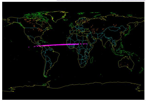
Three infrasound detectors just barely registered impact of 2014 AA. Each detector recorded the time of the event and knowing the speed of sound, the actual impact time could be computed. Then the distance from each station is computed and a circle drawn around each station.
