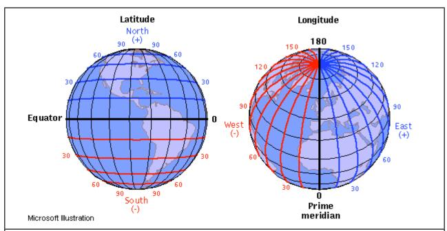
**Figure 1:** Latitude lines (left) trace "small circles" because the plane that contains them generally does not pass through the center of the sphere (earth, in this case). Longitude lines trace "great circles" because their containing planes do pass through the center of the sphere. (Illinois St. U.)
