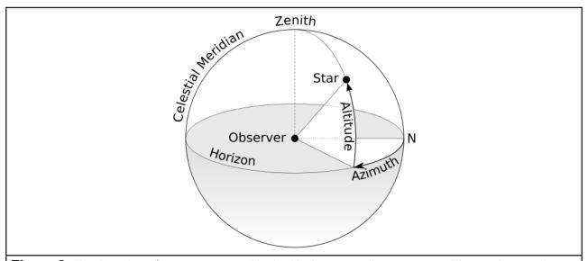
**Figure 2:** The location of a star measured in the Horizon coordinate system. The star's coordinates would be reported as its Altitude and Azimuth, which change as the earth rotates. (Wikipedia)
