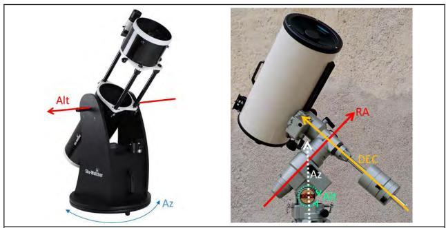
**Figure 4:** The two major types of telescope mounts. The left is an Altitude-Azimuth mount comprising a Dobsonian telescope. On the right is a German Equatorial mount that incorporates the ability to adjust the altitude and azimuth of the equatorial head (denoted by the Az and Alt labels).
