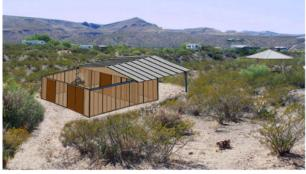
The proposed design for ASLC's Observatory includes a 16 x 20 foot roll-off roof and a 6 x 14 foot warm room.
