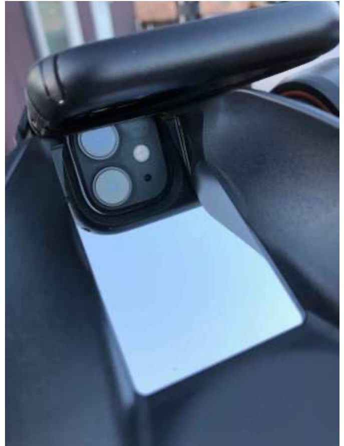
Smartphone camera lens positioned over the mirror which is directed at the sky.
