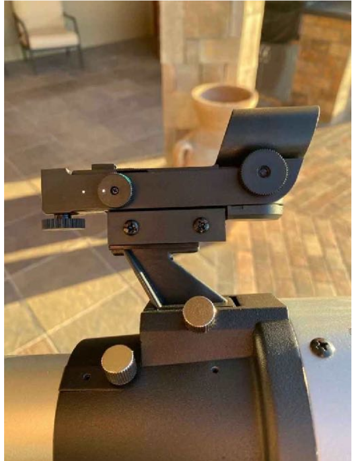
Red dot finder. The knob on the left facing front with the white dot is the on off. The one which sits underneath and the one on the right are for adjusting the finder position relative to the telescope.
