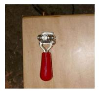
Azimuth engage lever
