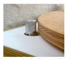
Azimuth roller disengaged
