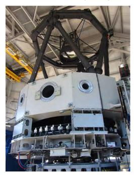
The Discovery Channel Telescope seen here inside its dome on Happy Jack Peak. This 170-inch reflector is a world-class research grade telescope just coming online this year.
