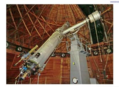
The 24-inch Alvan Clark refractor at Lowell Observatory. The dome around the telescope is made of local wood and supported by rubber tires to make the dome rotatable.
