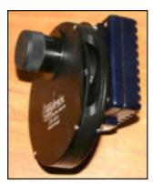
DSI Pro II with faceplate adapter and ATIK filter wheel
