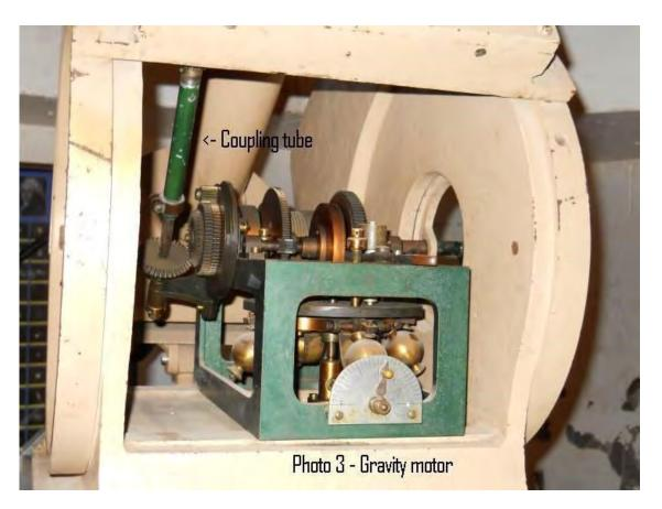
Sliding the green coupling tube upward engages its bevel gear with the mating gear and couples the gravity motor to the telescope. Look at the worm wheel sector. If it is not at the beginning of its travel, it should be rewound. See the description for this below. After the worm wheel sector is set to the beginning of its travel, slide the green coupling tube upward and tighten its clamp.
