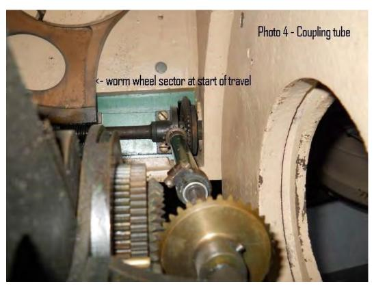
The photo shows the green coupling tube from inside the frame. The bevel gear pair at the bottom connects the gravity motor shaft from the fly-ball governor to the green coupling tube. The green coupling tube has another bevel gear at the top which engages with one above it on the worm shaft. Slide the tube upward until the bevel gears engage and tighten the clamp to keep it in place. The gravity motor is then coupled to the worm wheel sector which moves the telescope in right ascension.
