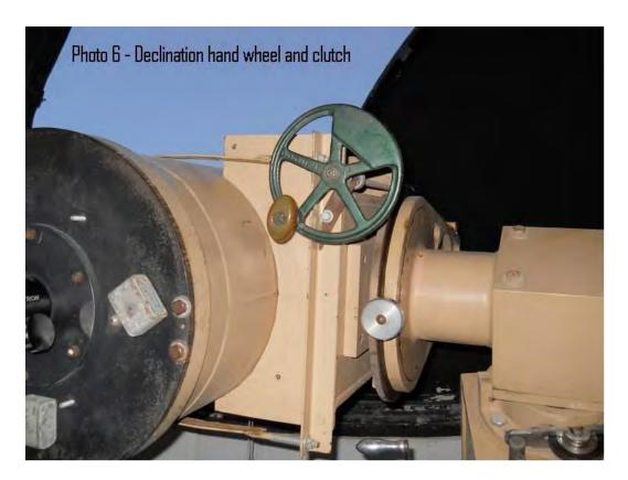
The declination hand wheel and clutch are shown above. The clutch locks declination movement to the hand wheel. The hand wheel allows fine movement, but may not be as convenient as loosening the clutch and pushing the optical tube where you want it. Retighten the clutch when done.
