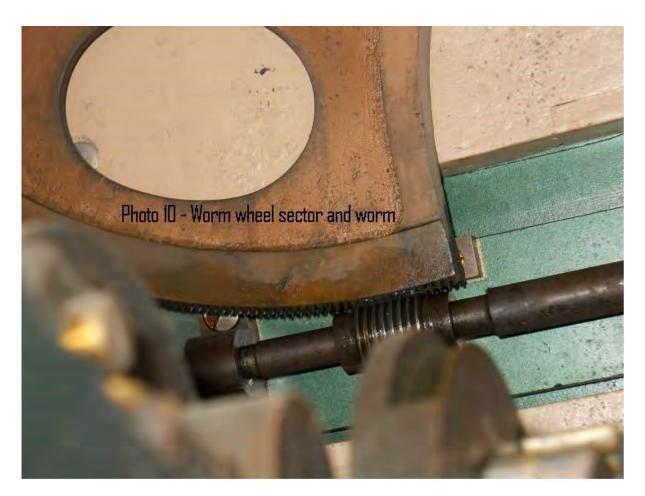
Turning the crank moves the right ascension worm wheel sector back to its starting point. The telescope will have to be moved back on target after moving the worm wheel sector. Reengage the motor by raising the green coupling tube until the bevel gears engage and tighten its clamp. The only thing to remember in moving the telescope is to keep the optical tube pointing above horizontal. Moving downward past horizontal may let internal mirrors move out of place.
