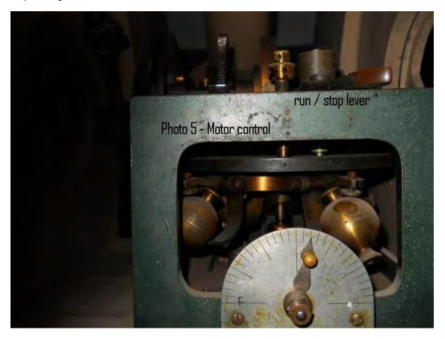
Move the lever on the top of the green housing to the left to start the gravity motor. The telescope should now be moving in right ascension compensating for the earth's rotation. The pointer above the scale marked F / S (fast / slow) controls tracking speed by adjusting the fly-ball governor. It needs to be adjusted for the type of target being tracked such as star, planet, or moon. It will require trial and error to find the right speed.
