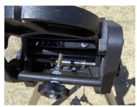
This follower yields an azimuth adjustment with very little slop. As you can see in this photo, it covers a much wider span of azimuth screw than the original, and exhibits almost no tilt when reversing directions.
