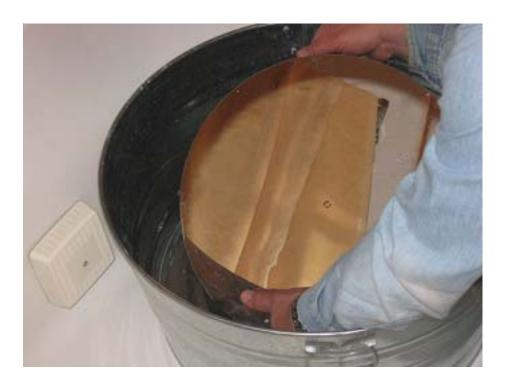
After thoroughly rinsing the mirror with warm tap water, it is time for hopefully, the final rinse.
