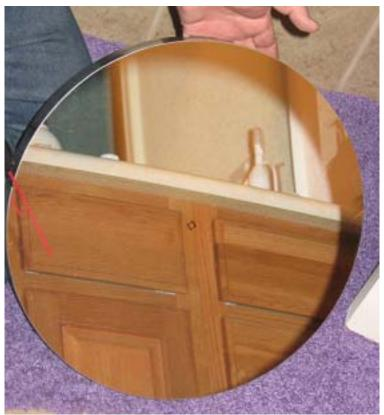
Chase the reminder of the water from the mirror surface with a can of compressed air, sometimes called Dust Off. Lowes again had this as did Best Buy. If after chasing all the water droplets off the mirror you see dried water spots on the mirror Rinse it again. This time use a mixture of 75% distilled water and 25% alcohol (denatured alcohol) Tequila is not an acceptable substitute. Then again chase the droplets off the mirror surface.
