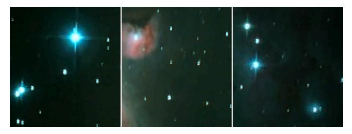
Satisfied with these images, I moved the imaging scope to be on Polaris, and recalibrated PHDGuide. As noted earlier, it took nearly twice as many RA steps to move the required 25 pixels, 17 steps compared to 9, but the calibration was successful. Then I took seven ten-minute images, the first is reproduced below. Again, there is noticeable image shift, I believe due to flex between guide and imaging scopes, but not any noticeable frame rotation.
