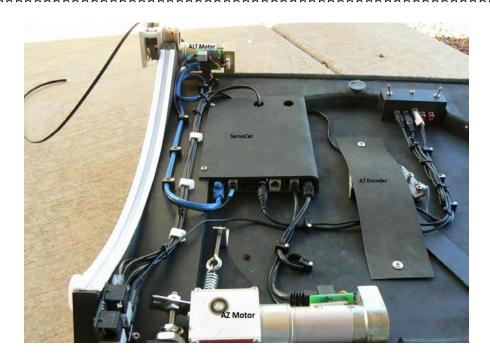
The system can track an object with good consistency depending on location in the sky. It clearly is not a match for an equatorial mount but I have tracked an object over one hour. Guiding is supported by the **ServoCat** but there is no practical way to mount a guide scope on the 18" UC. A Telrad is used for locating object areas. The tradeoff is tremendous light gathering but only for shorter intervals.
