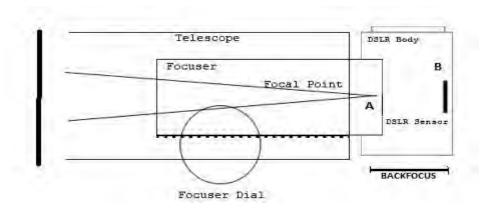
It required some research to determine the back-focus distance for the Canon EOS T1i. It required determining the distance from the image sensor to the middle of the bayonet flange. Also the T-ring adapter dimension has to be considered. It was determined that 44mm were required from the bayonet flange to the image sensor and another 12 mm was required for the T-ring adapter. All together about 2.25 inches of back-focus was necessary.
