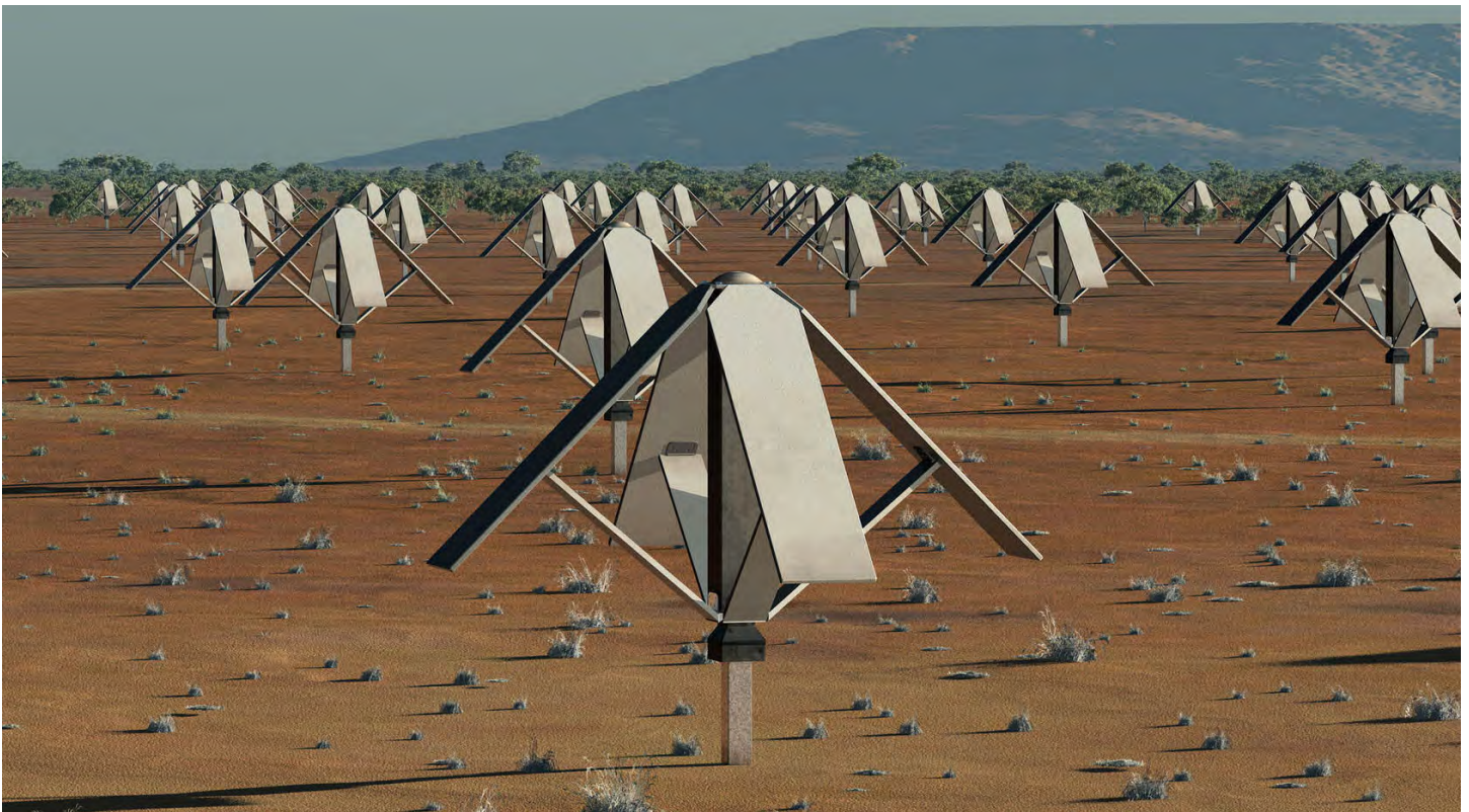
Figure 3: Phased Array. For low frequency radio telescopes, a phased array of simple dipole antennas will pick up signals in the 50 to 350 MHz frequency range. This array will be built in Western Australia. These antennas actually consist of two dipoles at right angles. A dipole is a simple antenna made of a conductor that is half the wavelength of the desired signal. The dipole is cut in the middle and the two feed wires are connected to two sides of the dipole to feed the signal to the receiver.
