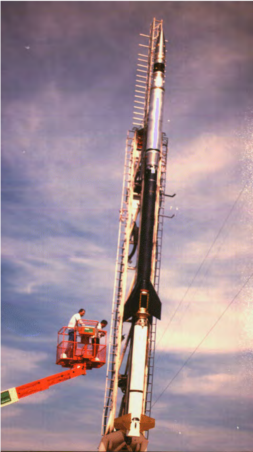
Figure 5: MSSTA. The Multi-Spectral Solar Telescope Array (MSSTA) is inside its stainless steel protective skin (the silvery section at the top of the missile). Below the telescope is the Black Brant sustainer stage and at the bottom is the Terrier solid rocket booster. This assembly is NASA sounding rocket 36.049 at White Sands Missile Range, in May 1991. The MSSTA array is composed of fifteen telescopes designed to observe the Sun in ultraviolet and soft x-rays.
