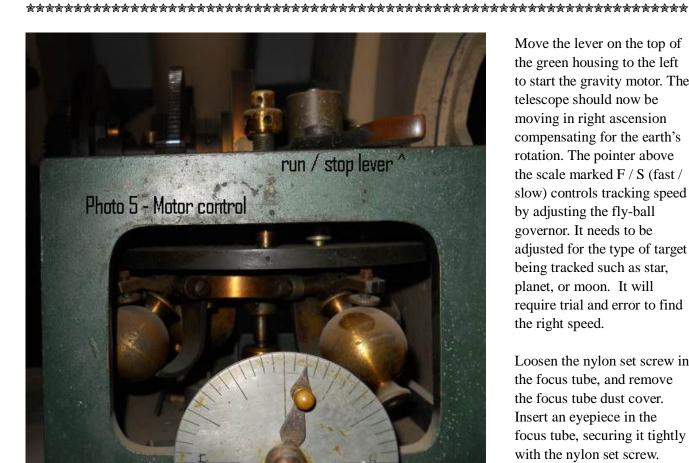
Move the lever on the top of the green housing to the left to start the gravity motor. The telescope should now be moving in right ascension compensating for the earth's rotation. The pointer above the scale marked F / S (fast / slow) controls tracking speed by adjusting the fly-ball governor. It needs to be adjusted for the type of target being tracked such as star, planet, or moon. It will require trial and error to find the right speed.
