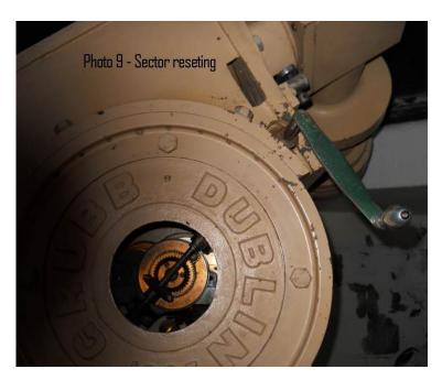
If the worm wheel sector has reached its end of travel, disengage the motor by loosening the clamp on the green coupling tube. Then remove the crank from its square pin, placing it on the square pin on the opposite side as shown above. Turn the crank clockwise while facing it. This will turn the worm and move the worm wheel sector back to its starting point.
