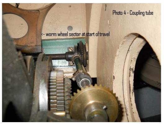
This shows the green coupling tube from inside the frame. The bevel gear pair at the bottom connects the gravity motor shaft from the fly-ball governor to the green coupling tube. The green coupling tube has another bevel gear at the top which engages with one above it on the worm shaft. Slide the tube upward until the bevel gears engage and tighten the clamp to keep it in place. The gravity motor is then coupled to the worm wheel sector which moves the telescope in right ascension.
