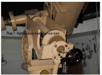
The right ascension hand wheel and clutch are on the back side of the mount. The clutch is at the top and may be difficult to reach. The right ascension hand wheel moves the telescope faster than the declination hand wheel. It is harder to set to a precise position. Again, it can be disengaged and pushed. Retighten the clutch when done.
